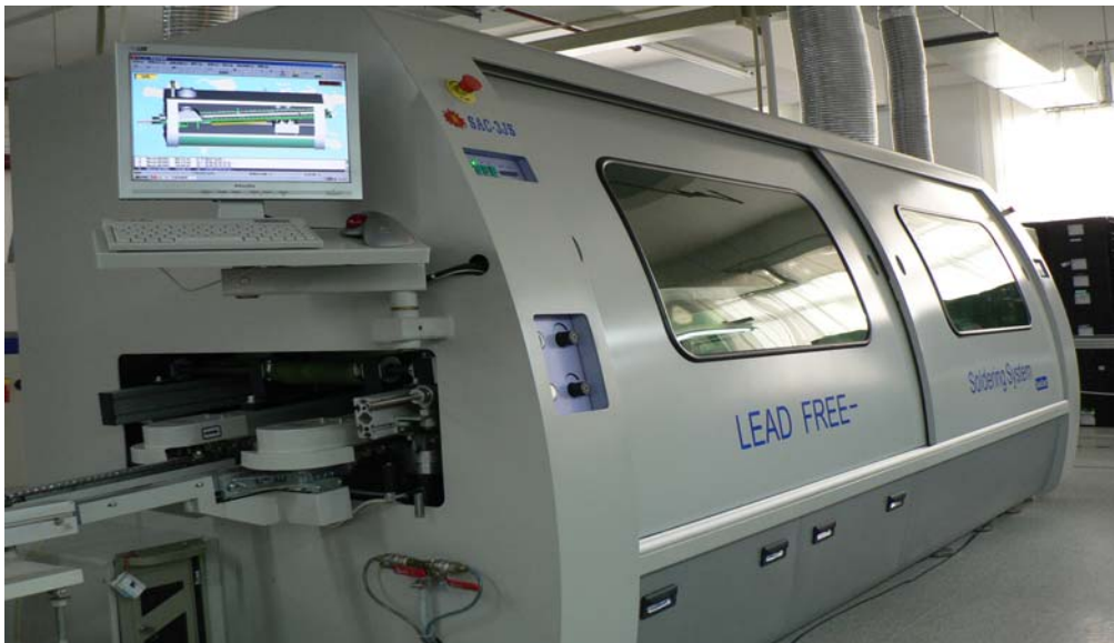
Lead Free Reflow Soldering Machine in Jan Yin Chan Shenzhen, China May/2005
